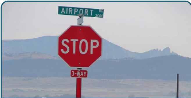
Example of a stop sign with a red reflective post panel
