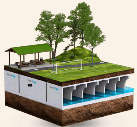
Infiltration Gallery (source: StormTrap.com)
